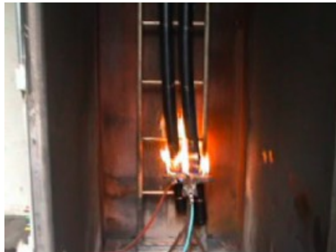
Figure 7. Fire test of high voltage cables
